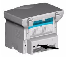
The power cord is used as a 230 V power unit cut off. As a precaution,
